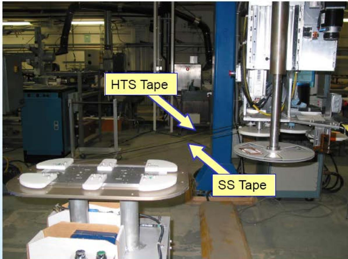
*A coil being wound with a computer controlled winding machine*
