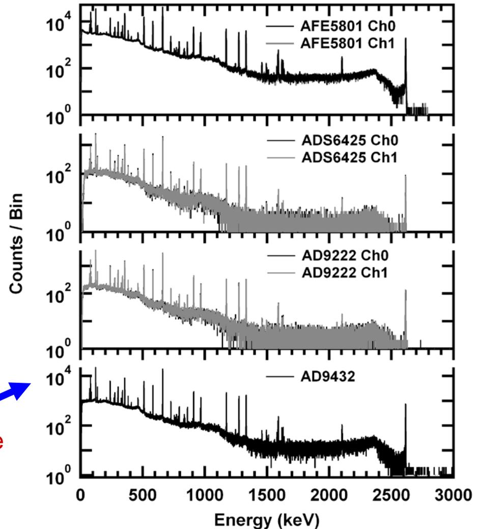
Energy spectra from a 40% coaxial HPGe Detector and multiple radiation sources
