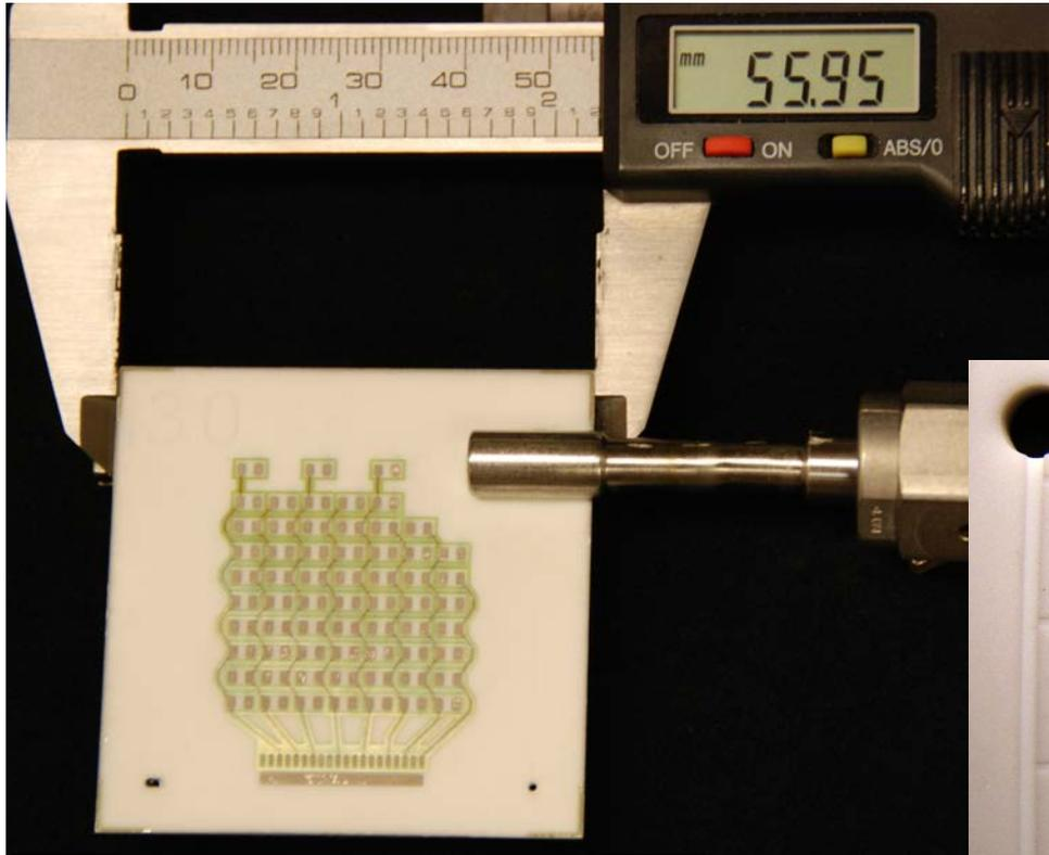
Bottom Side – quench resistor for each pixel.
