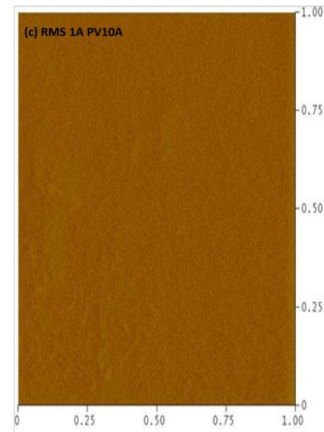
RMS roughness reduction by 1 order and optical flatness reduction from 1.6 micron to 0.5 micron with Sinmat's Reactive CMP (RCMP) polishing, (b) AFM picture of standard polish showing fractured surface (RMS 20A, (Peak to Valley) PV 90A) and (c) AFM picture of RCMP surface shows atomic smooth surface (RMS 1A, PV 10A).
