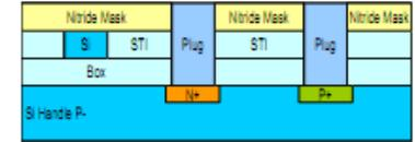
7) Protect silicon nitride is removed and devices are reinserted into standard CMOS7 processing
