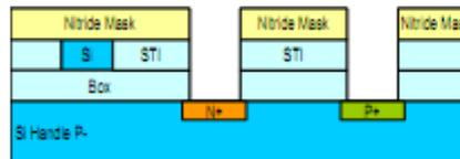
6) Polysilicon deposition into NBOX CUT and PBOX CUT areas followed by CMP (Chemical Mechanical Polish)
