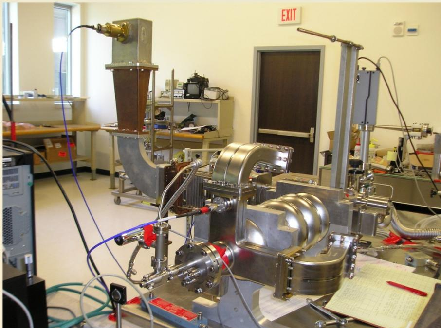
5-cell cavity test set up
