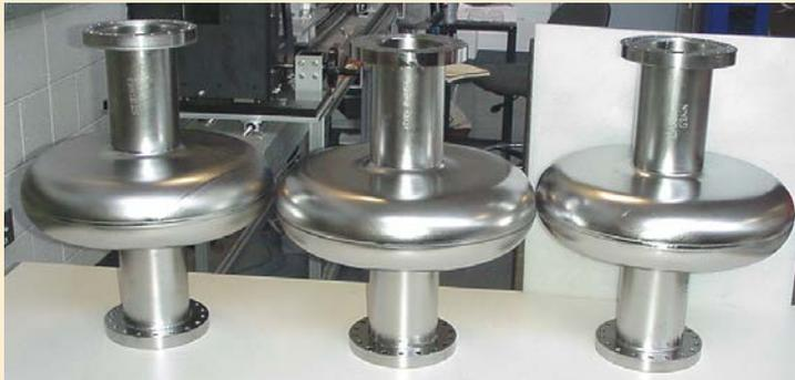
Three 650 MHz test cavities
