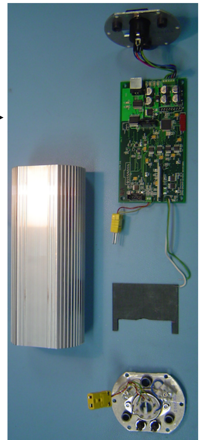
STRAW Control Box Disassembled (optic plate not shown)
