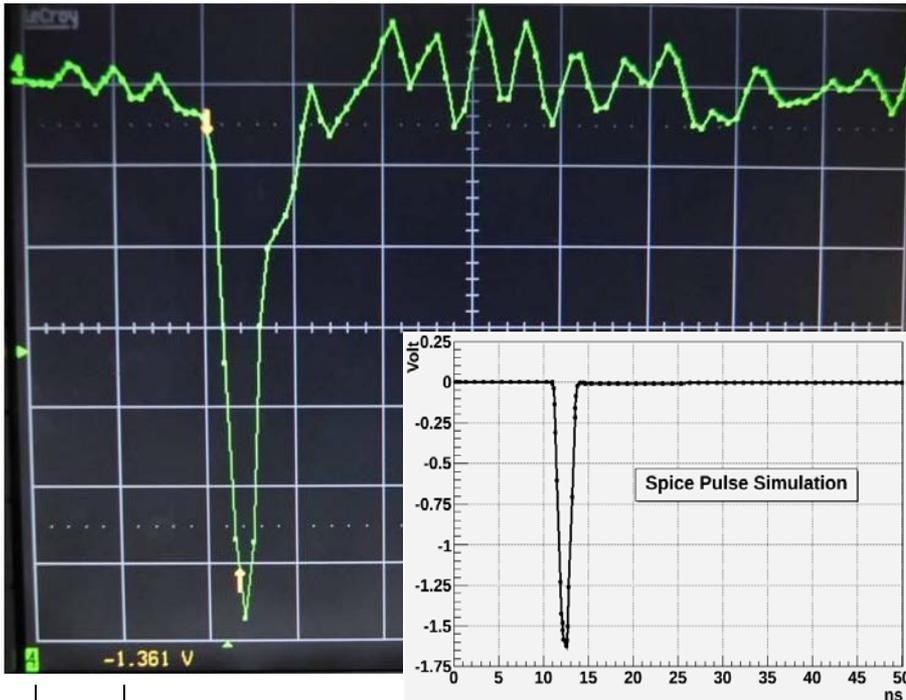
← Pulse from **Xe filled panel in 2003**, tested **2010**, 1.0 mm electrode pitch.
