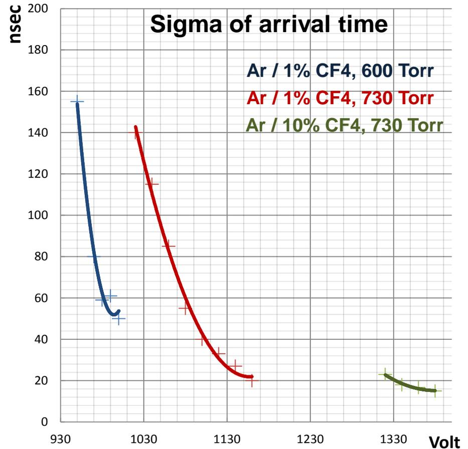
Gas mixtures & pressures working at **higher voltage** ➡ **faster timing**
