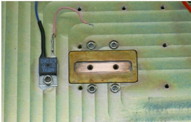
Transistor heat spreader mounted to aluminum housing.
