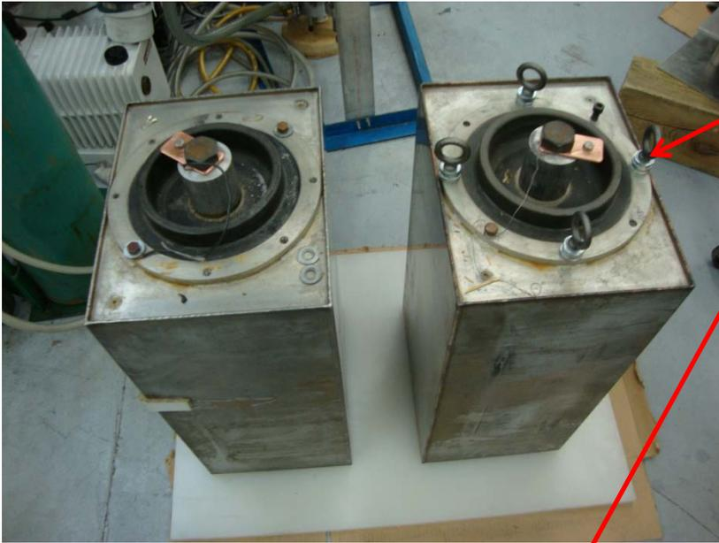
3 $\mu$ F, 60 kV capacitors to be connected in series
