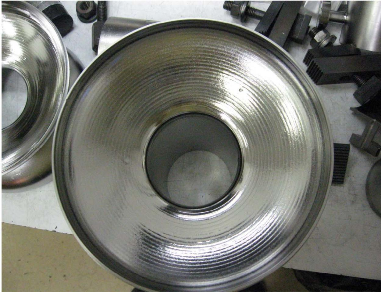
The beam parameters were: 40 mA, 0.5mm diameter beam, travelling at 18 inches per minute, the melting diameter is about 6 mm with a circular pattern at 10 kHz.
