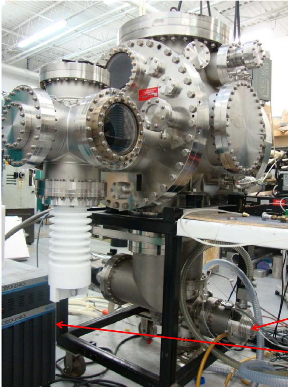
Chamber reaches  $3 \times 10^{-8}$  Torr with test cathode, anode, high current and voltage feedthrus.
