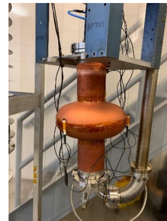
RDT-10 1.3 GHz Nb 3 Sn cavity
