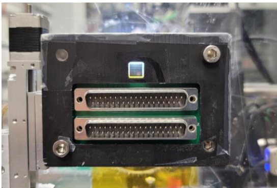
Innovative Carbon (size: 5.2 mm x 5.2 mm x 0.07 mm and pitch: 100 μm)
