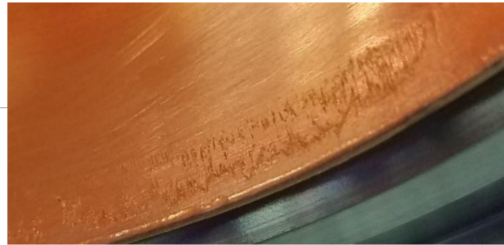
A photograph showing striations in plating attributed to a leak in a seal during the plating process (Figure from Ref. [1]).
