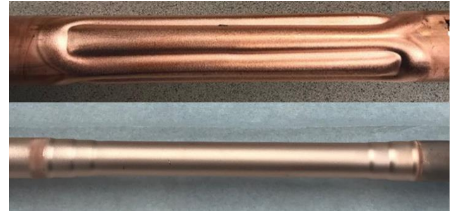
Erosion patterns for the stationary (top) and rotating (bottom) serpentine magnet packs.
