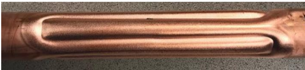
Erosion pattern produced by the serpentine magnet pack
