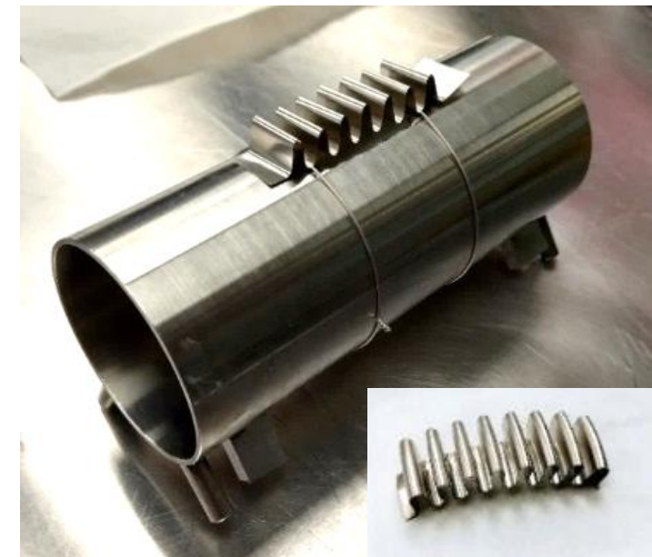
The sample holder used for this work loaded with a corrugated test coupon. (Inset) An LCLS-II bellows section.
