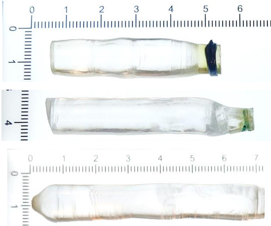
Optimized high-purity transparent \beta -Ga 2 O 3 crystal grown after parameter optimization.
