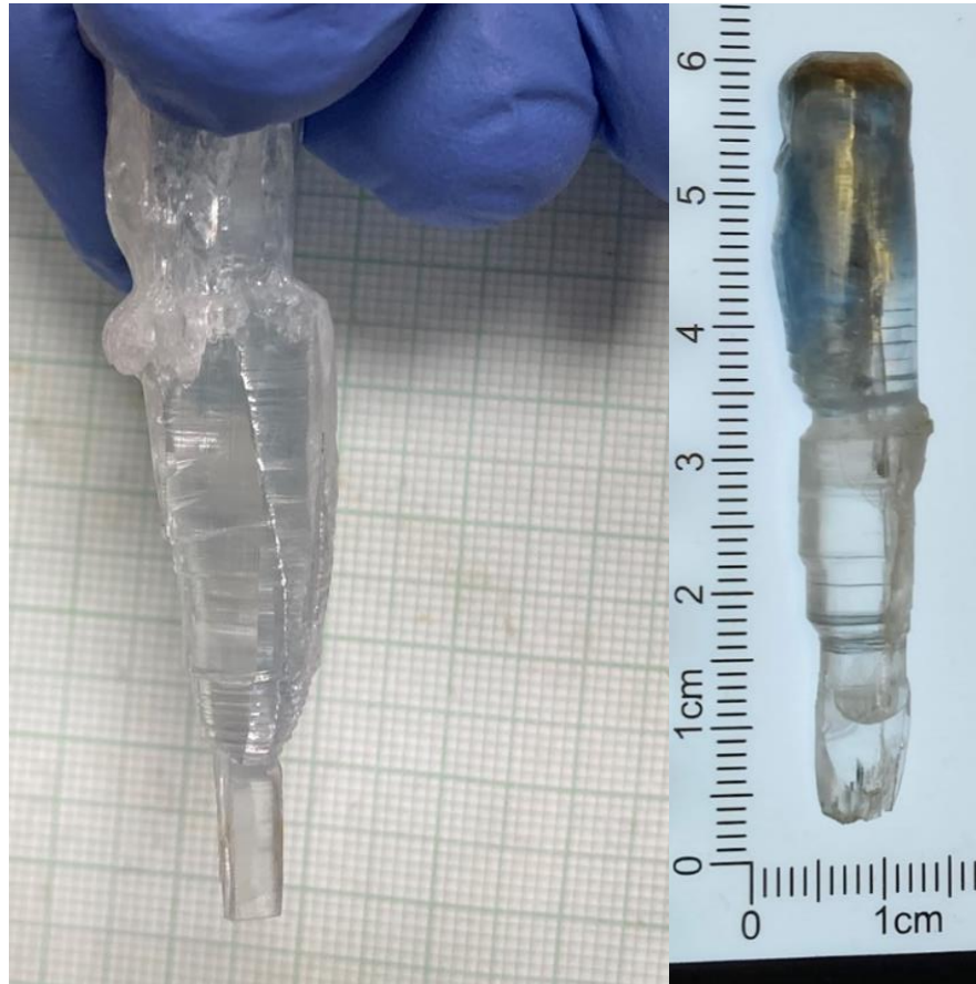
Yb 3+ (left) and Nd 3+ (right) doped \beta -Ga 2 O 3 crystals growth using OFZ technique.
