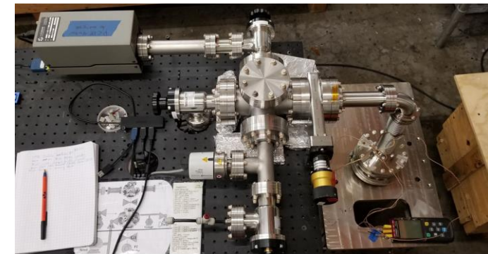
Outgassing test: rate of rise Q = 6E-7 mbar L/s
