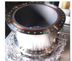
BNL LDRD three high power 308mm ID BLAs Technology: Shrink fit SiC (Coorstek SC-35)
