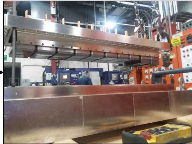
Lowering tile/backer flange assembly into housing
