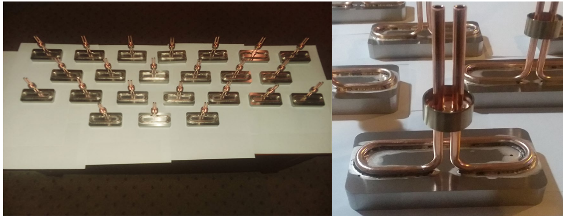
Backer/Cooling Tube Assemblies (without SiC tiles)
