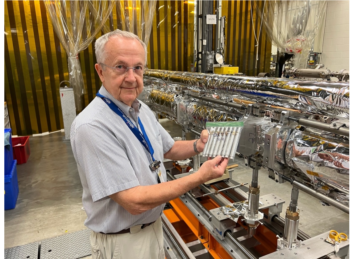
George Biallas prepping for installing BNNT cartridges on C100 cryomodule
