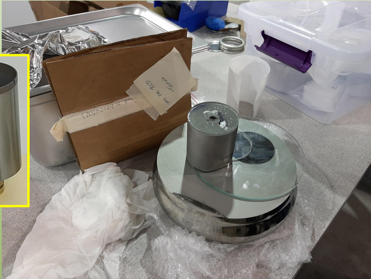
Practice slab of non-detector grade HPGe
