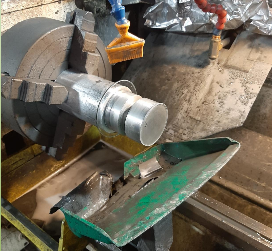
60 mm x 60 mm cylinder V-Groove cut on lathe
