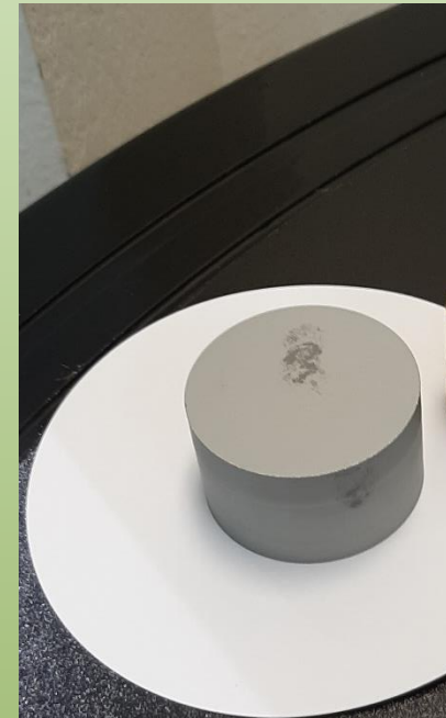
60 mm x 60 mm cylinder core-drilled from the slab
