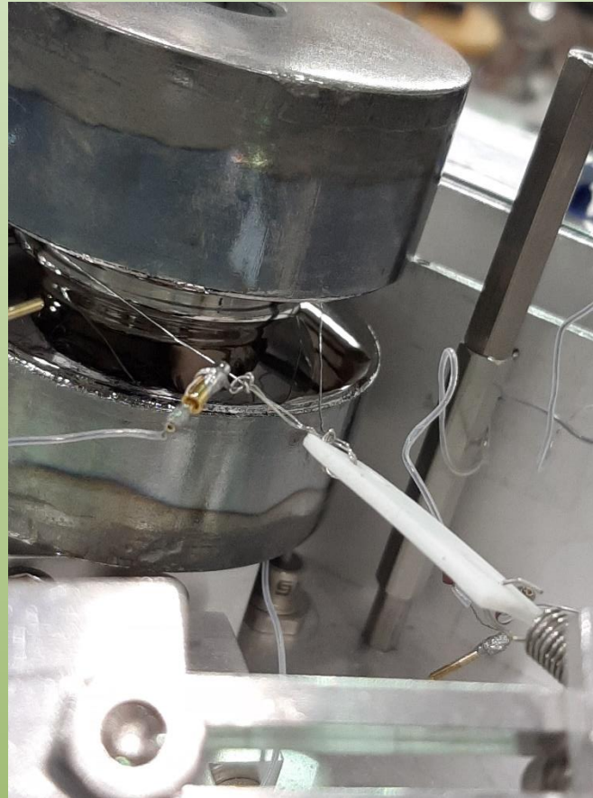
Spring loaded wire loop on ring contact. This is the signal contact
