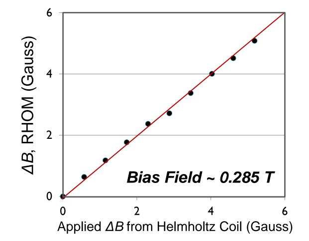
Calibration-free determination of magnetic field
