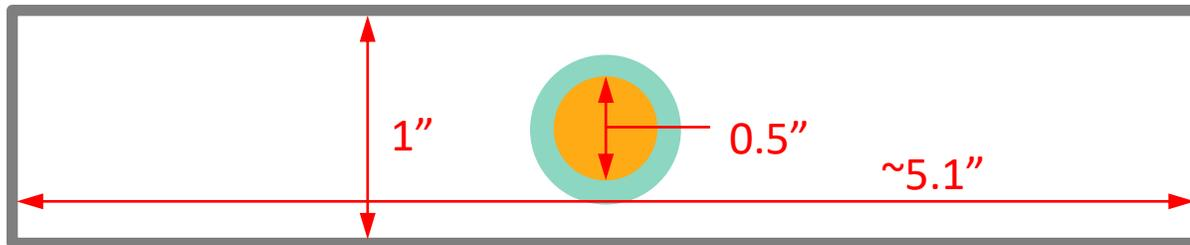
*The low internal clearance and high aspect ratio of the CEBAF waveguide structure present difficult technical challenges.*
