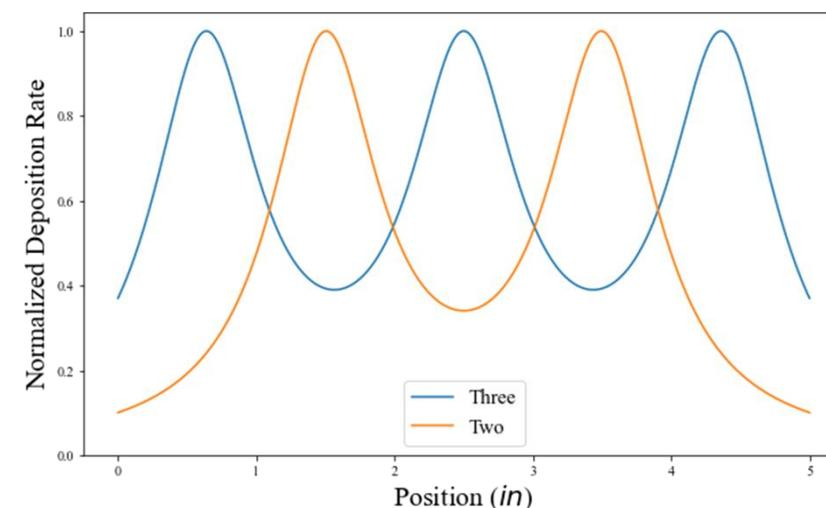
*Normalized deposition rates for two- and three-magnetron configurations, assuming the fit parameters from the trial in the above image. The addition of a 3<sup>rd</sup> magnetron is needed to reduce the azimuthal variation in film thickness.*
