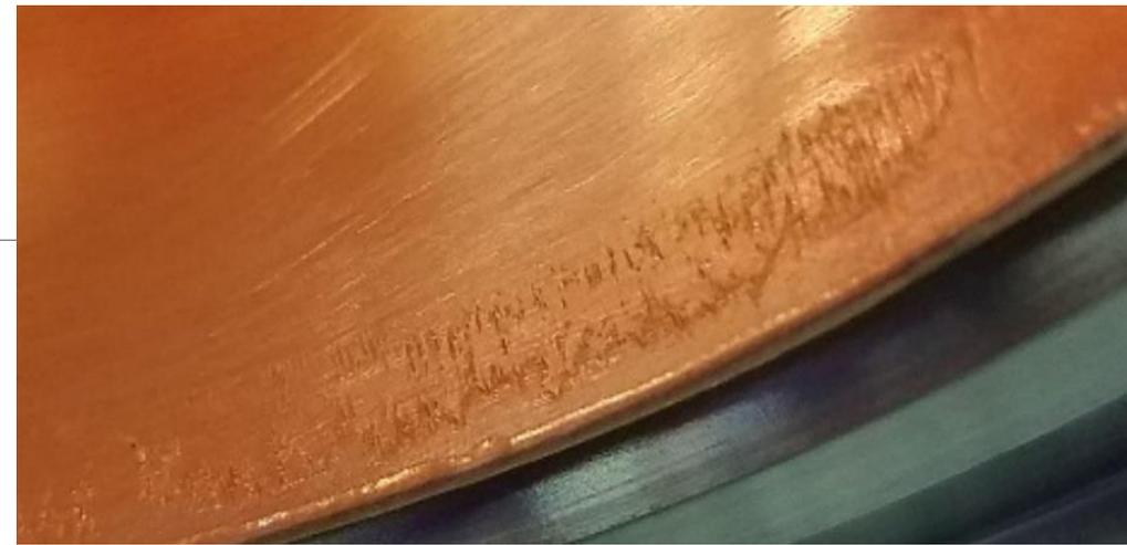
A photograph showing striations in plating attributed to a leak in a seal during the plating process (Figure from Ref. [1]).
