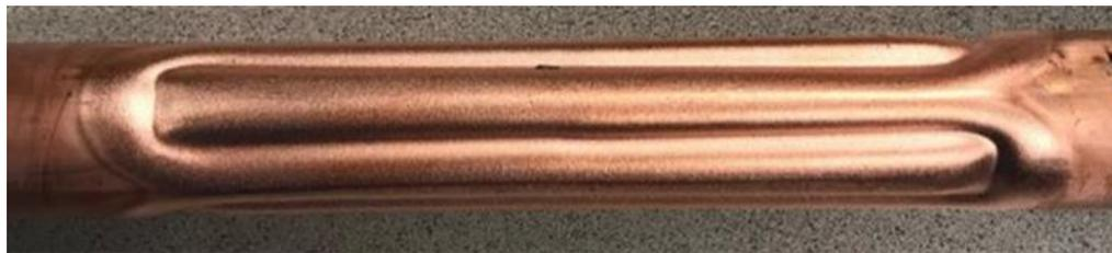
*Erosion pattern produced by the serpentine magnet pack*
