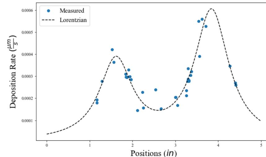
*Deposition rate measurements taken at many points along the length of the sample holder along with a double-Lorentzian fit.*
