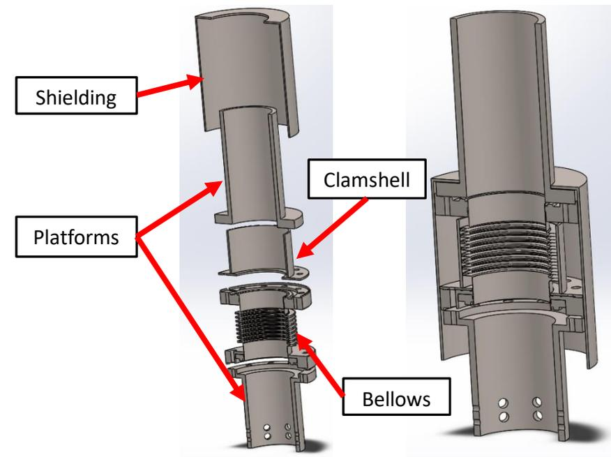
The design for the LCLS-II sample holder. The design is all stainless-steel; its primary functions are mechanical support and shadow shielding.
