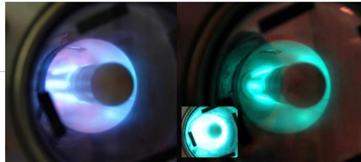
*The radial magnetron shown during an in-situ plasma clean step (left) and during a Cu deposition (right) with a reduced exposure time setting on the camera. The inset image is of the same Cu deposition step without any reduction in exposure time.*
