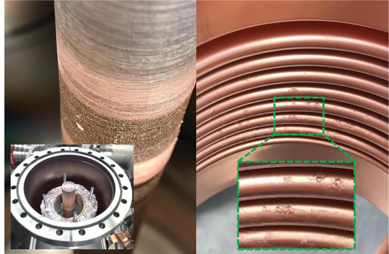
(Left, inset) Fixturing used for the LCLS-II bellows included UHV aluminum foil. Flaking was observed on the foil and nearby on the magnetron itself (shown left), above the active region. (Right) The resulting film on the LCLS-II bellows. (Right, inset) A close-up of what turned out to be dense, solid metal ‘bumps’ in the Cu coating.
