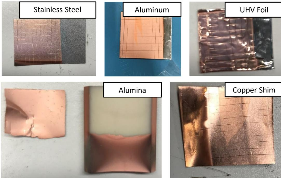
Photographs of films deposited on test coupons to determine acceptable masking/fixturing materials.
