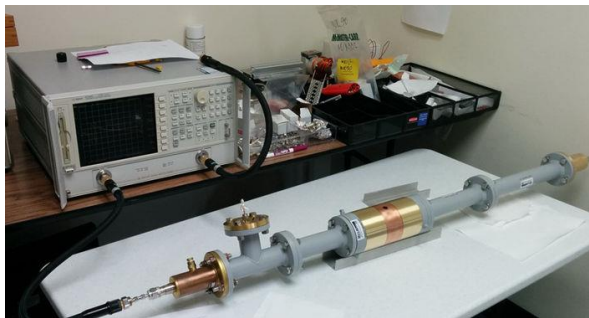
Fast ferroelectric 400 MHz tuner successfully tested at CERN
