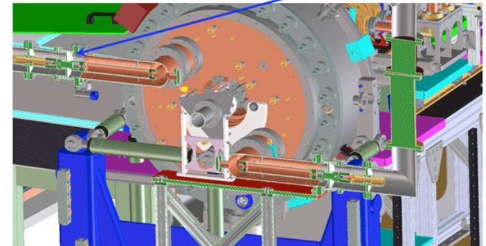
Example: the Advanced Photoinjector Experiment's VHF gun in the LCLS-II injector. Window broke: charging because of the direct line of sight for the beam. A new 90-degree coupler will keep ceramic vacuum window out of harm's way
