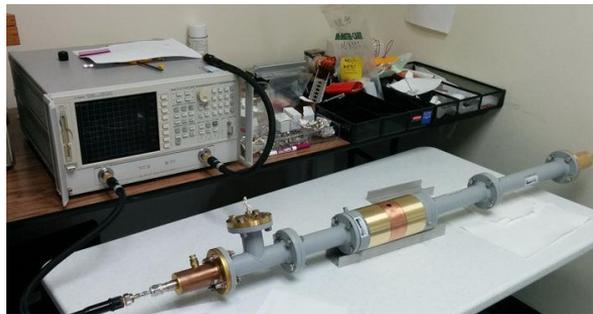
Fast ferroelectric 400 MHz tuner
