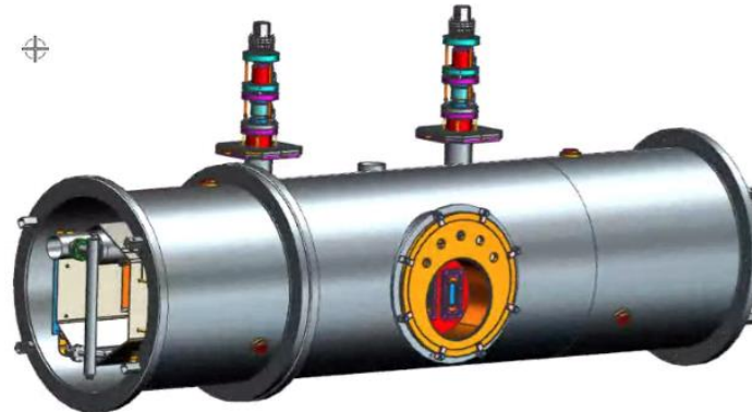
C100 cavities with thermal shield
