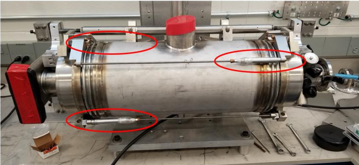
C100 cavity with two of four BNNT C100 cartridges shown during test assembly with location of third cartridge indicated.
