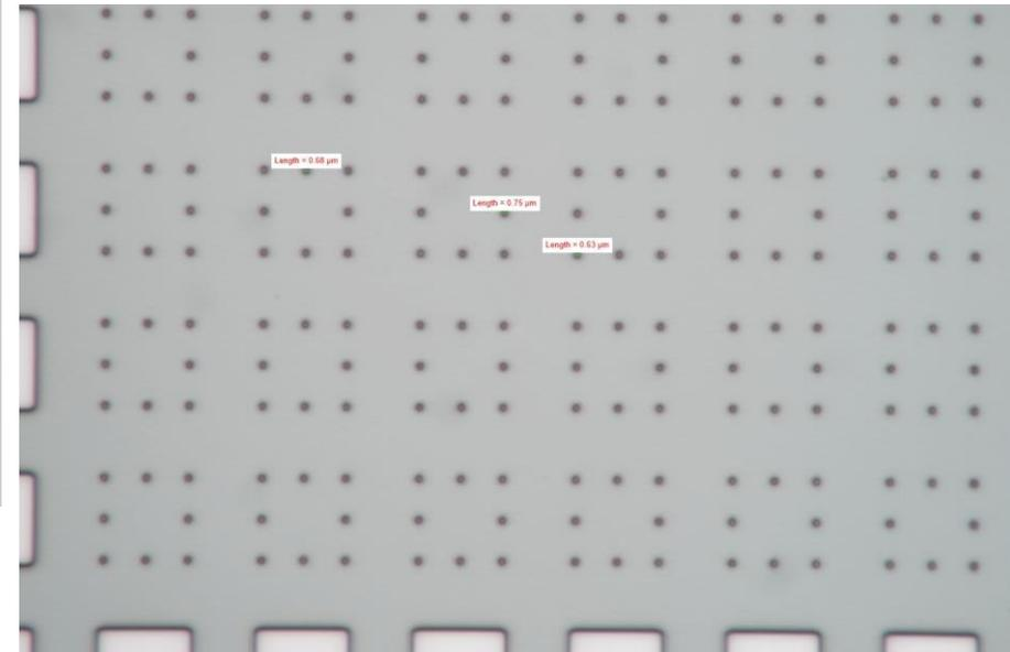
FPA section before metal contact deposition
