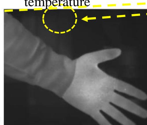
The circled area shows the defective pixels recovered after temperature circling.
