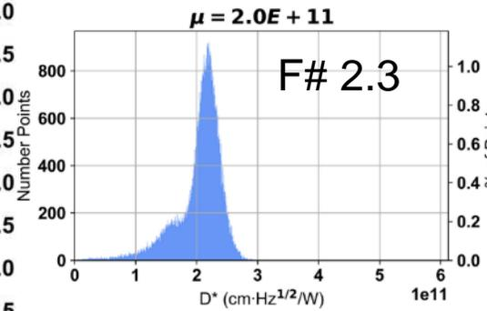
Although median D\* was unchanged, the high noise tail side split into a separate peaks.
