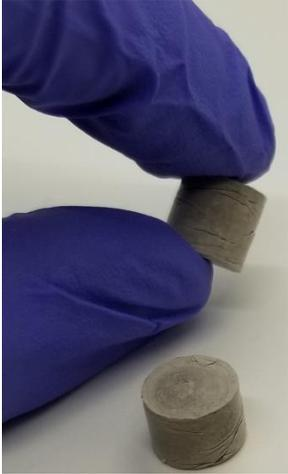
BNNT pellets are fabricated from compressed refined BNNT material.
