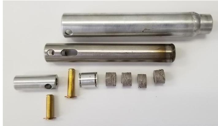
Multiple BNNT pellets are combined in a cartridge to provide required spring constant and compressive damping.
