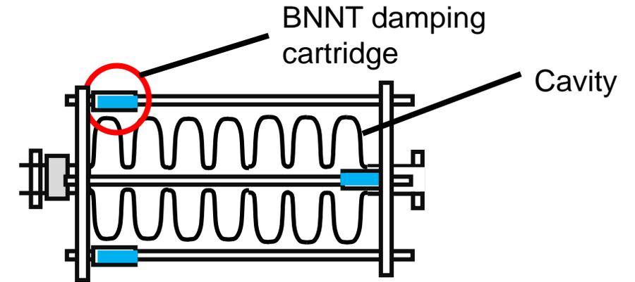
Four cartridges of BNNTs (three illustrated) provide passive vibration damping of length oscillations of the C100 SRF cavity.
