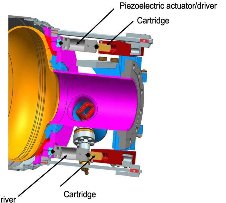
BNNT pellet installed onto an LCLS-II cavity. Standard parts (A) are readily exchanged for BNNT cartridge holders (B). BNNT cartridge holder components (C) prior to assembly. BNNT cartridge (D) is circled in red installed on a LCLS-II cavity between the tuner plate and piezoelectric actuator.
