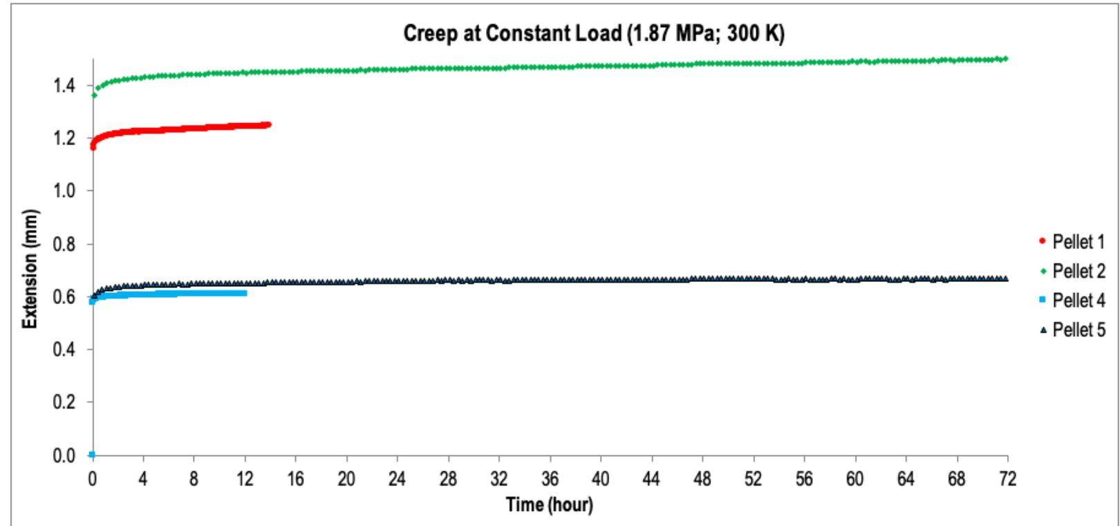
Preliminary creep measurements show that most of the BNNT pellet creep is within 4 hours but there is a tail in the creep that extends for several days. Additionally, cycling average pressure and temperature on the pellets introduces some creep. Current measurements are investigating temperature and pressure cycling.
