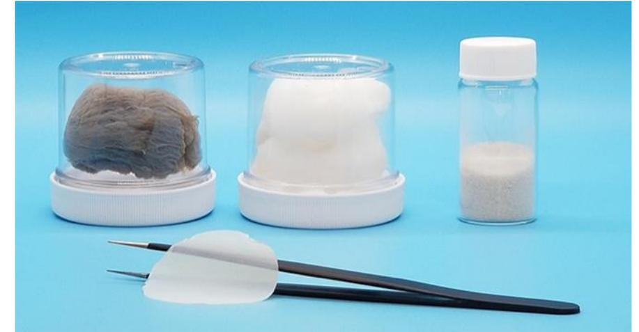
As-synthesized puffball (left); refined puffball (center), powder (right); buckypaper (bottom)
