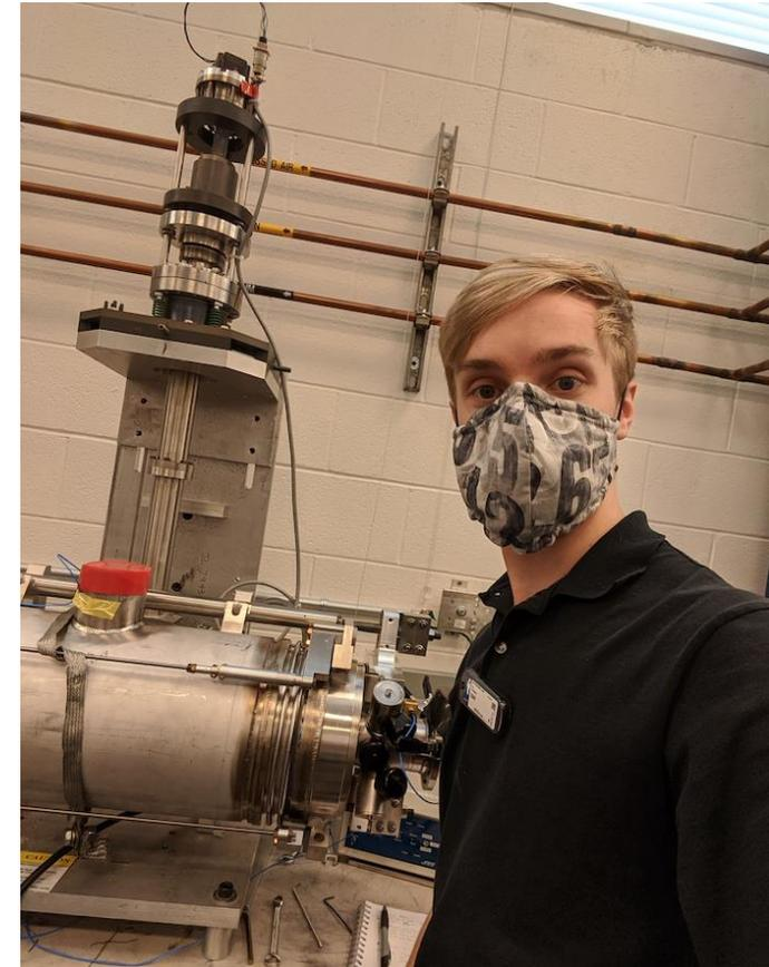
C100 cavity tuner drive mechanism behind and above cavity used to compress the cavity to achieve resonance frequency.
