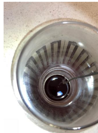
Puck melted in Pt crucible
