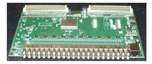
High density digitizer: **32 channels** Kintex-7 1G Ethernet at wire speed 10G under development
