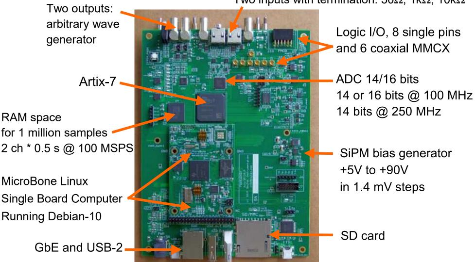
Two inputs with termination:  $50\Omega$ ,  $1k\Omega$ ,  $10k\Omega$
