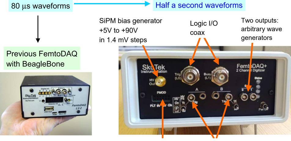
Logic I/O, 8 pins Arranged as PMOD Two inputs:  $50\Omega$ ,  $1k\Omega$ ,  $10k\Omega$ 14 or 16 bits, 100 MSPS
