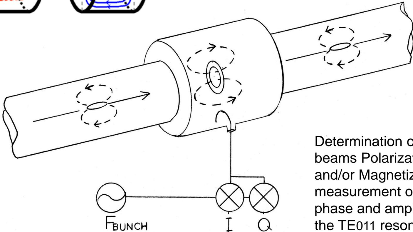
Determination of the beams Polarization and/or Magnetization by measurement of the phase and amplitude of the TE<sub>011</sub> resonance induced.
