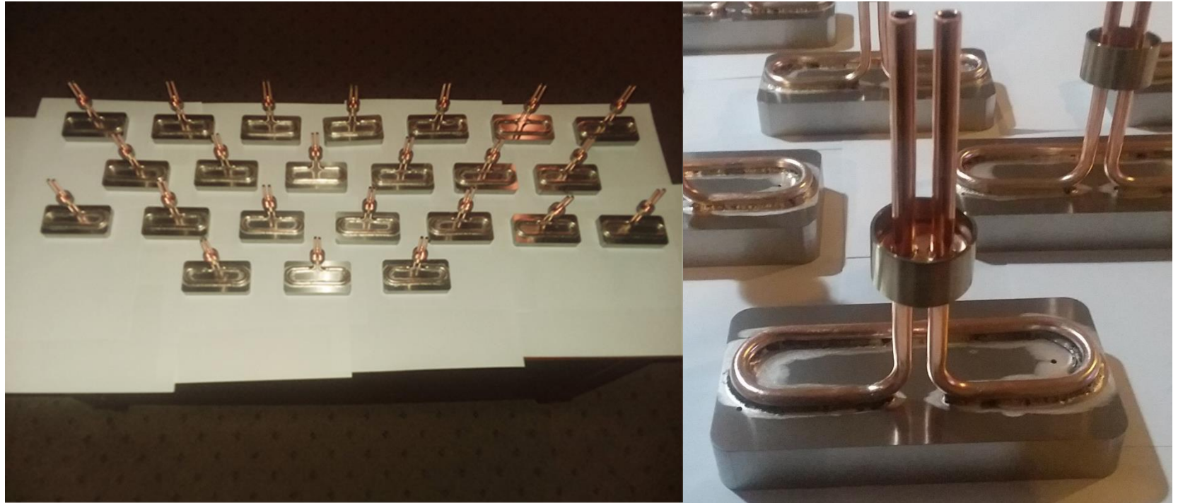
Waveguide Backer Assemblies (without SiC tiles) Extra assemblies are for Ceramic joining tests
