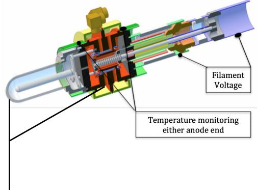
Thread a thermocouple into the water channel to monitor the temperature closest to the vane tip to prevent damage during 2000C operation of the filaments in the oven at the end of bakeout.
