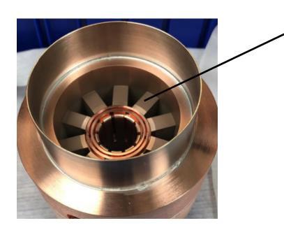
Note that the copper plating was not thick enough for subsequent brazing operations, but is adequate for the next level of assembly and operation of the prototype. Ready for holes to be drilled into the vanes for the antenna connection
