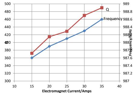
Resonant frequency and Q of anode with G-810 ferrites in two diametrically opposite ferrite cavities vs electromagnet current. Unloaded Q was 526
