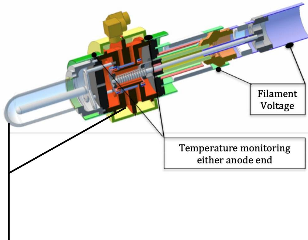
**Thread a thermocouple into the water channel to monitor the temperature closest to the vane tip to prevent damage during 2000C operation of the filaments in the oven at the end of bakeout.**
