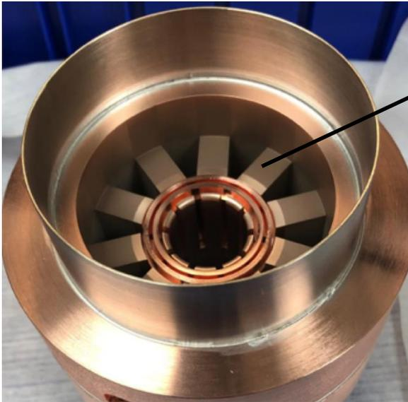
Ready for holes to be drilled into the vanes for the antenna connection
