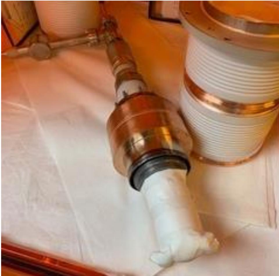
Leak tight assembly after repair for a machining operation that put a hole in one of the water channels to vacuum.
