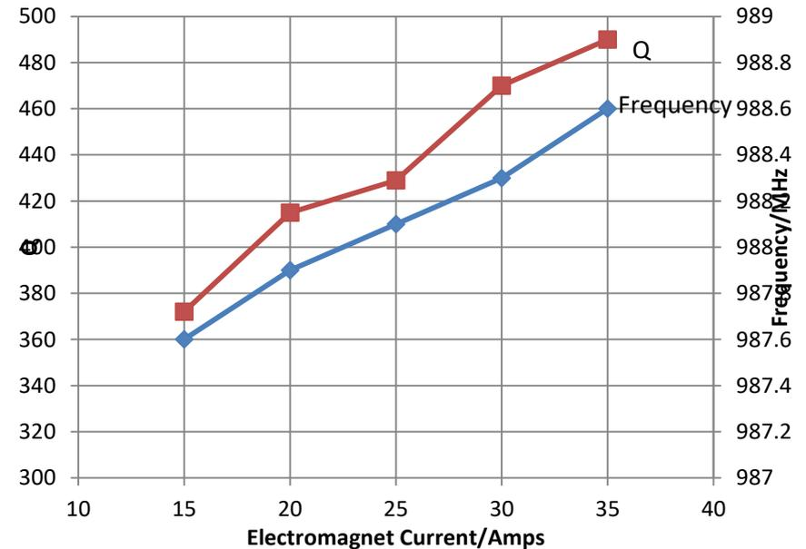
Resonant frequency and Q of anode with G-810 ferrites in two diametrically opposite ferrite cavities vs electromagnet current. Unloaded Q was 526
