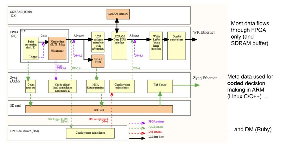
Various "Data Flow" options, can also simply output all data from FPGA and sort out offline
