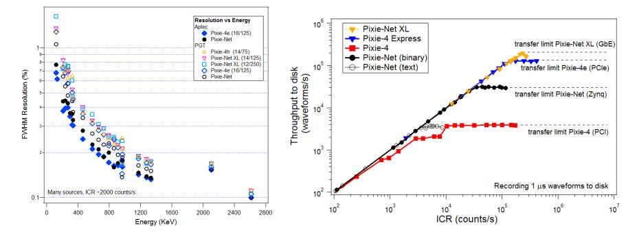
Pixie-Net XL HPGe energy resolution: matching older readout electronics.
