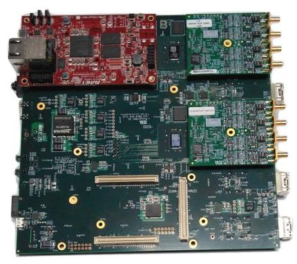
Main board with ADC daughtercards and Zynq controller module card stack
