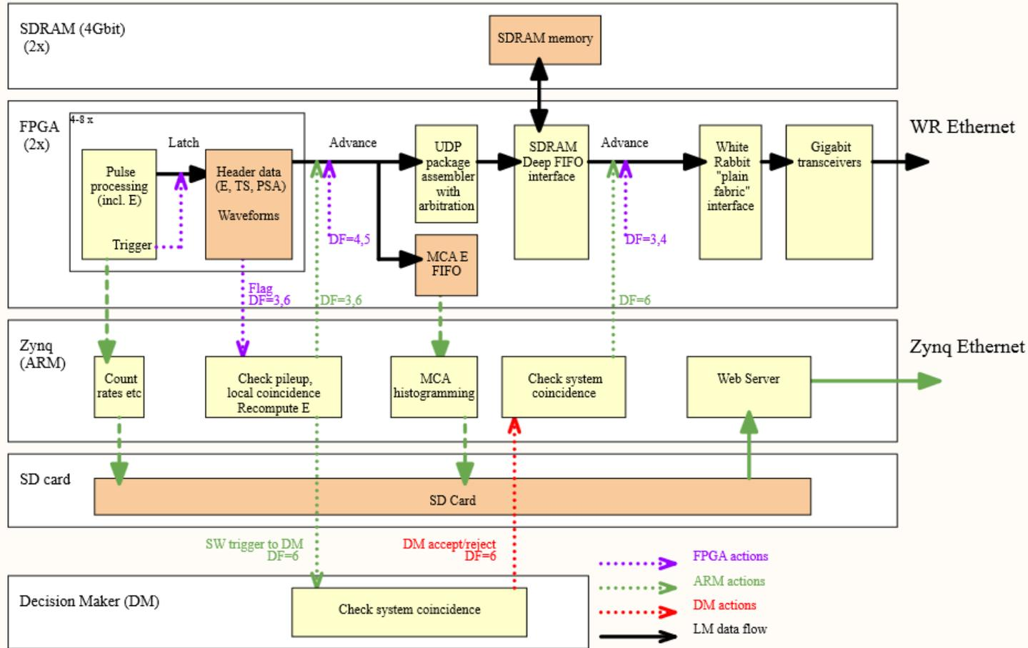
Most data flows through FPGA only (and SDRAM buffer)
