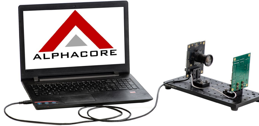
200kfps Camera Prototype and Test Target
