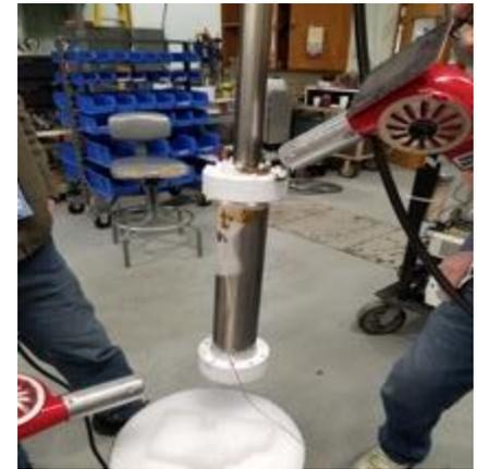
Setup for thermal cycling test sample is at the end of the crane line about to be inserted into the cryogenic Dewar
