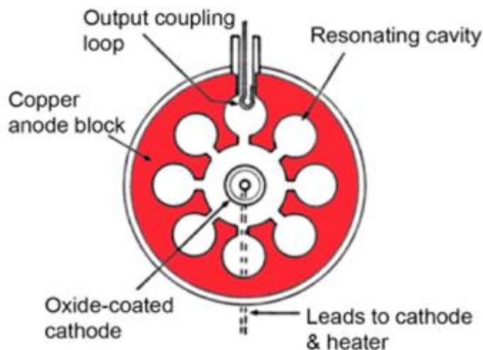
Resonant cavity magnetron high-power high-frequency oscillator
