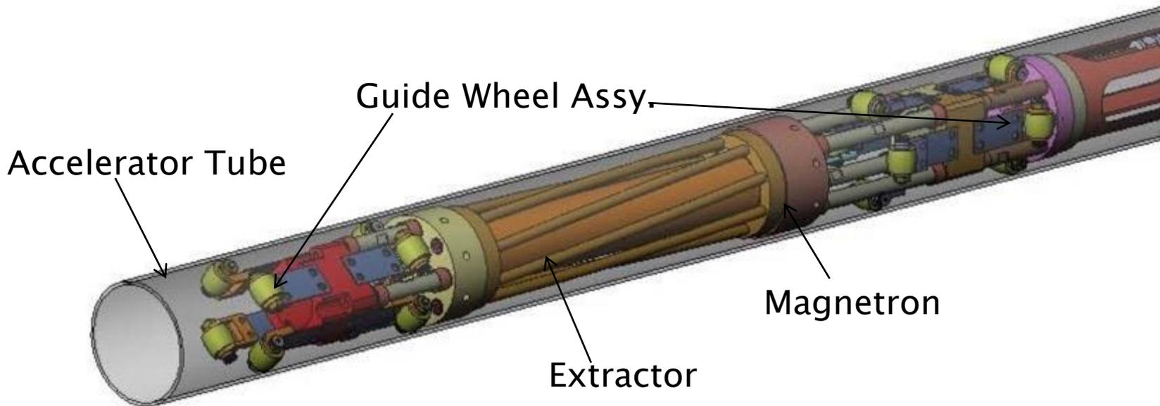
Integrated IAD Cathode Sputtering Magnetron in
