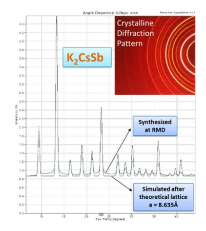
A key enabler is the RMD's patented process for synthesizing "bulk" K<sub>2</sub>CsSb material
