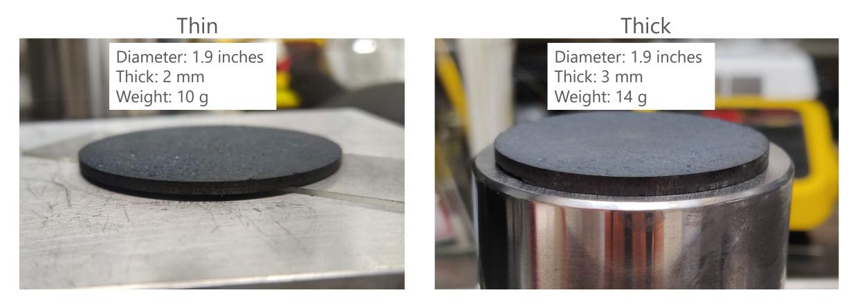
• To improve target robustness: Strain > 10,000 psi, Post-press anneal at 100 C
