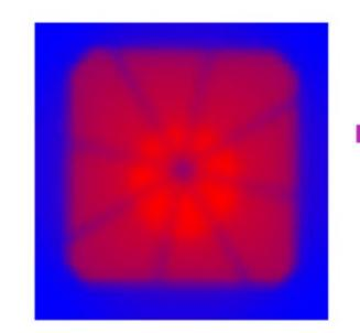
405 nm LED photoemission map ⇒ 16.4 % QE @ Al passivated region (24% on #1) ⇒ ~ 10% on SS
