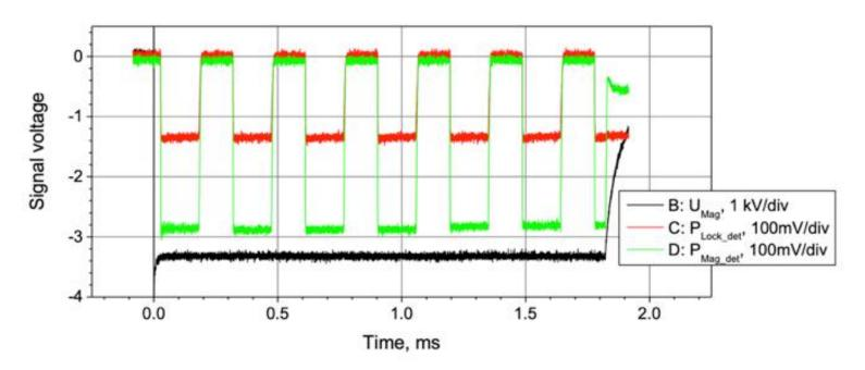
The black trace shows the magnetron voltage (1 kV/div), The red trace shows the detected locking signal of  $\approx$ 100 W, The green trace shows the magnetron output detected signal of  $\approx$ 330 W.
