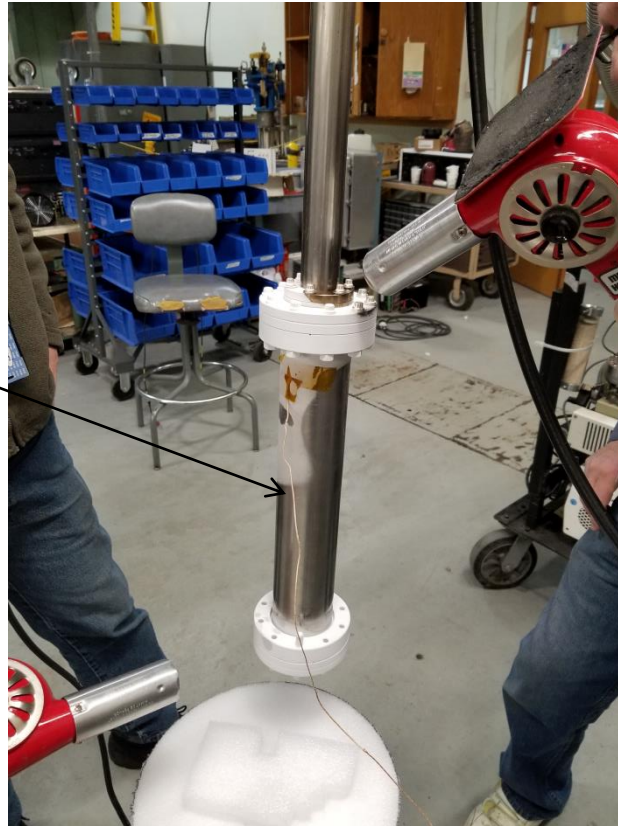
Photo showing test sample pulled out of Dewar and being warmed up
