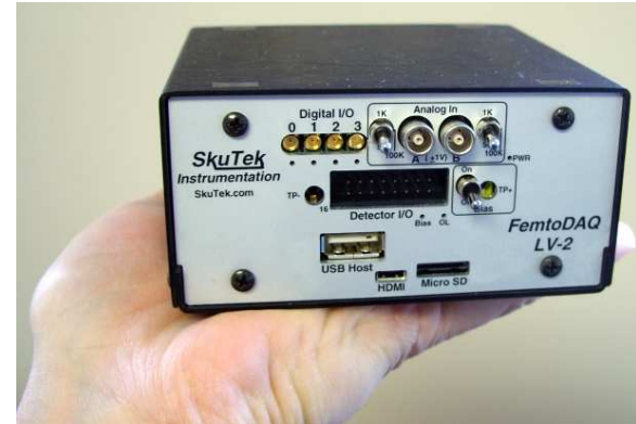
Low cost networked digitizer (2 channels)
