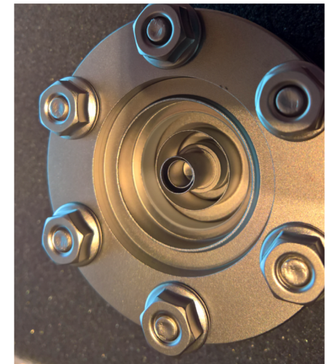
Back of Cathode as received
