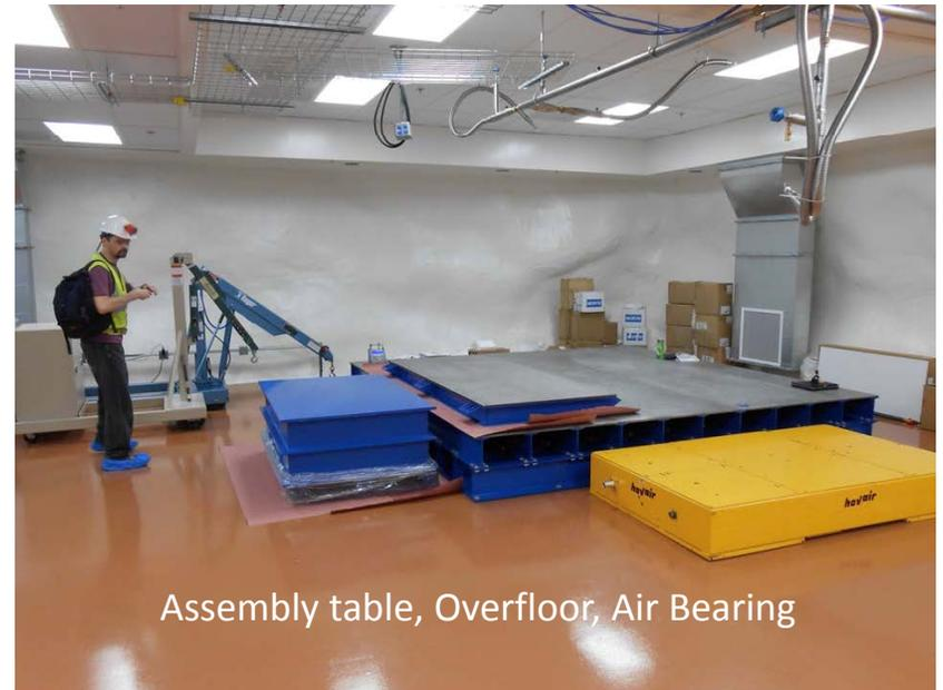
Assembly table, Overfloor, Air Bearing
