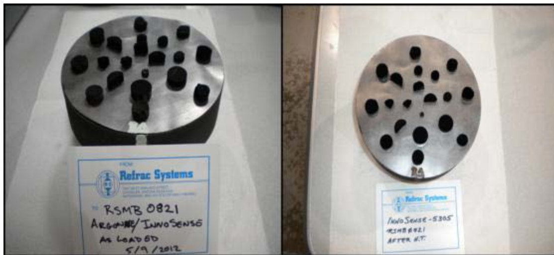
C-aerogels before (left) and after (right) vacuum heating
