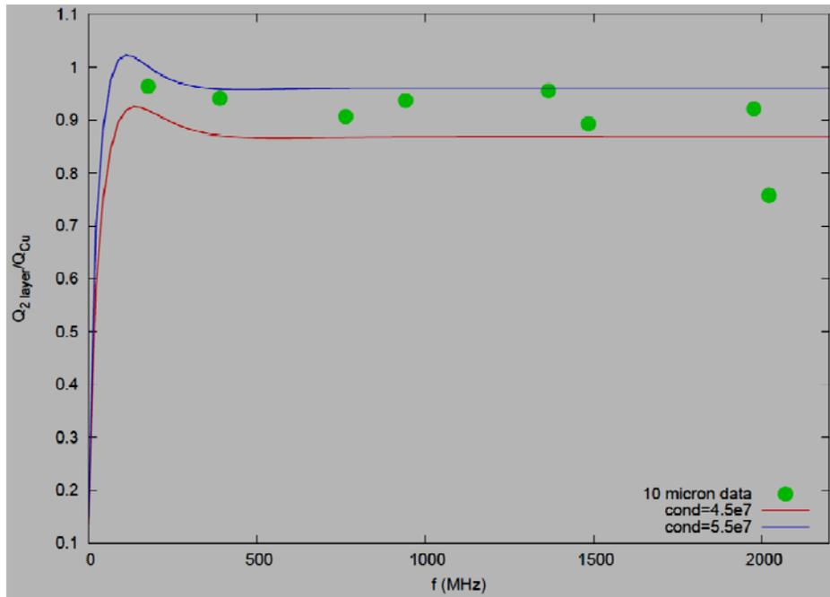
Ratio of resistivity to bulk copper vs. frequency
