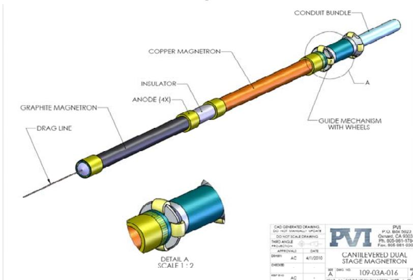
***Concept of a plasma deposition device based on staged magnetrons***
