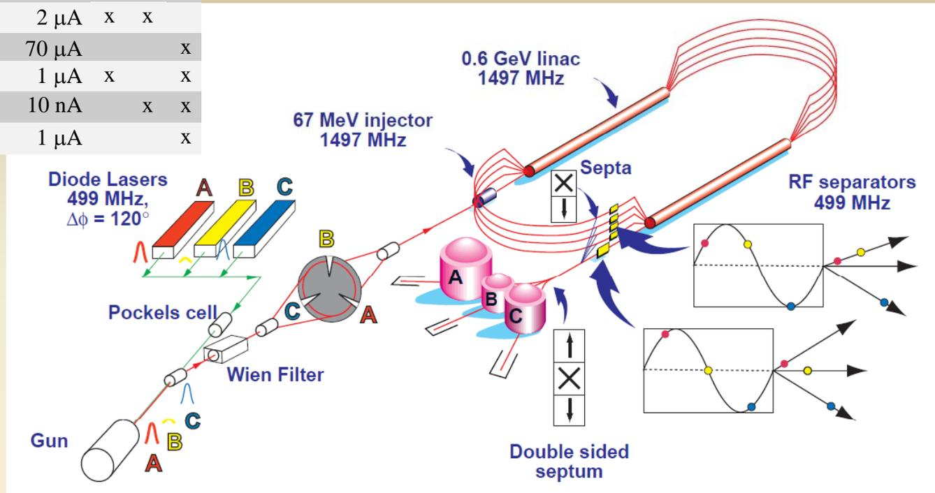
First large **high-power CW recirculating e-linac** based on **SRF** technology
