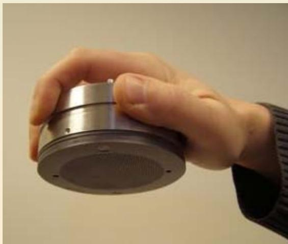
**"Gamma Puck":** Handheld detector with tungsten shell and tungsten collimators
