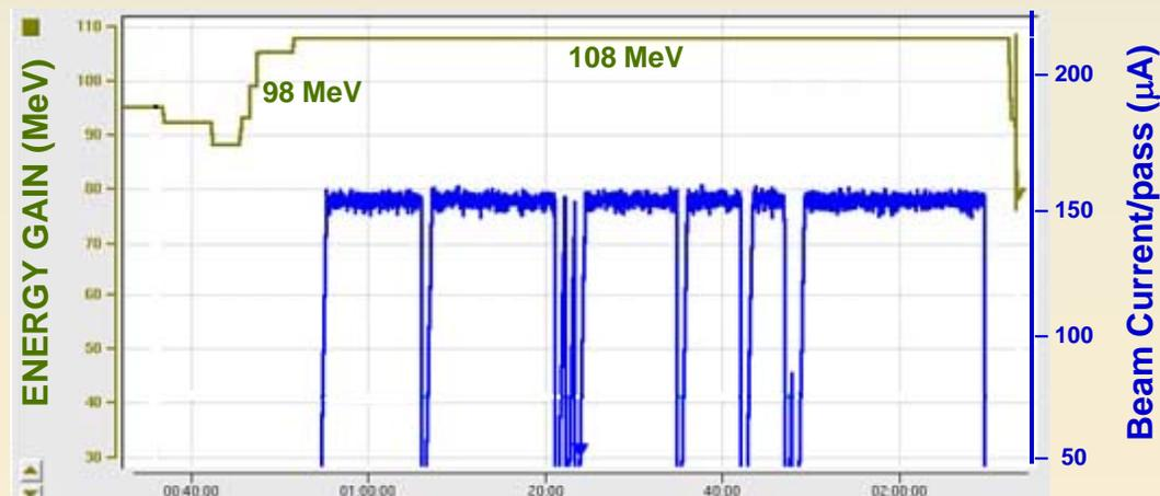
C100 reached design energy gain (108 MeV) for the nominal 12 GeV current of 465  $\mu$ A on May 17 2012.
