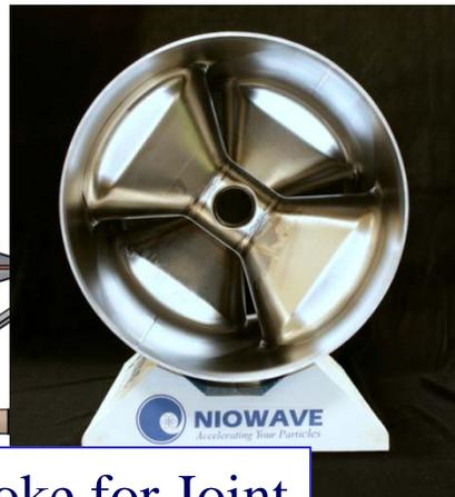
700 MHz Double Spoke for Joint Technology Office (DOD)
