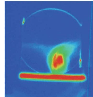
High brightness photoelectron beam image on YAG scintillator.
