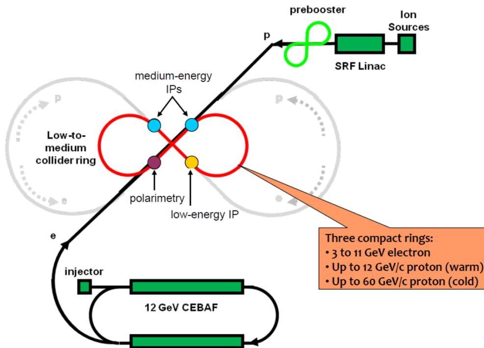
Reaching the luminosity of the designed machine will require crab cavities to collide the beams head-on while preserving the crossing angle at the interaction point.
