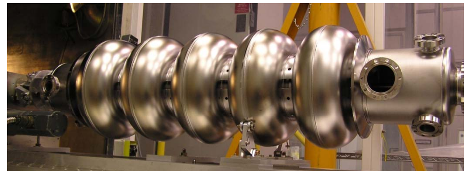
Stony Brook U designed, AES built high-current cavity
