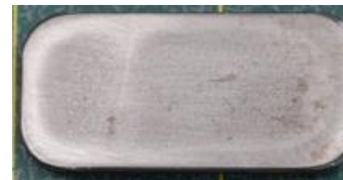
FAST SiC small tile + CVD BN encapsulation coating + CVD W backing plate (shown)
