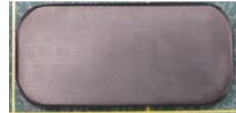
FAST SiC small tile + CVD BN encapsulation coating
