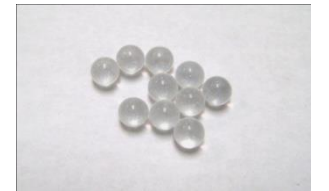
FB-CVD coated with \text{Ti}_{0.5}\text{Si}_{0.5}\text{O}_2
