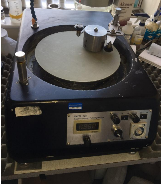
Polishing machine with customized fixture for 45 mm cubes.
