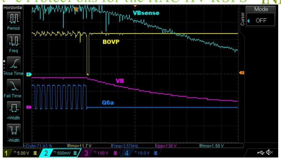
Expanded (i.e., zoomed in 10 times) waveforms shown in previous slide for OVP testing including the tripping and subsequent shutdown of the main switching circuit that drives the rest of power supply Time base is 1 ms/division.
