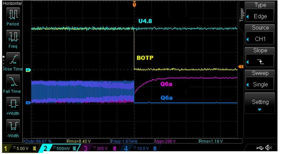
Overtemperature protection (OTP) tripping which turns off the gate to the main switching circuits which, in response, turns off the output voltage of the extremely high voltage power supply. Time base is 10 milliseconds (ms) per division.
