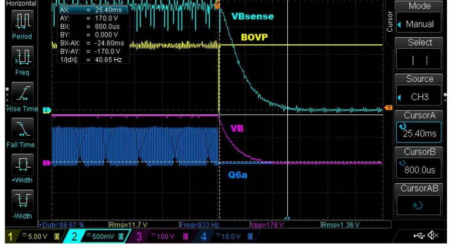
The waveforms over voltage protection (OVP) testing including the tripping and subsequent shutdown of the main switching circuits that drives the rest of the power supply Time base is 10 milliseconds (ms) per division.
