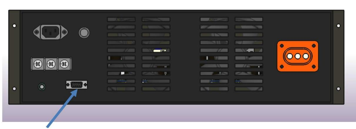
Interlock, remote control and monitor signals (in general, customized for specific customer end use.
